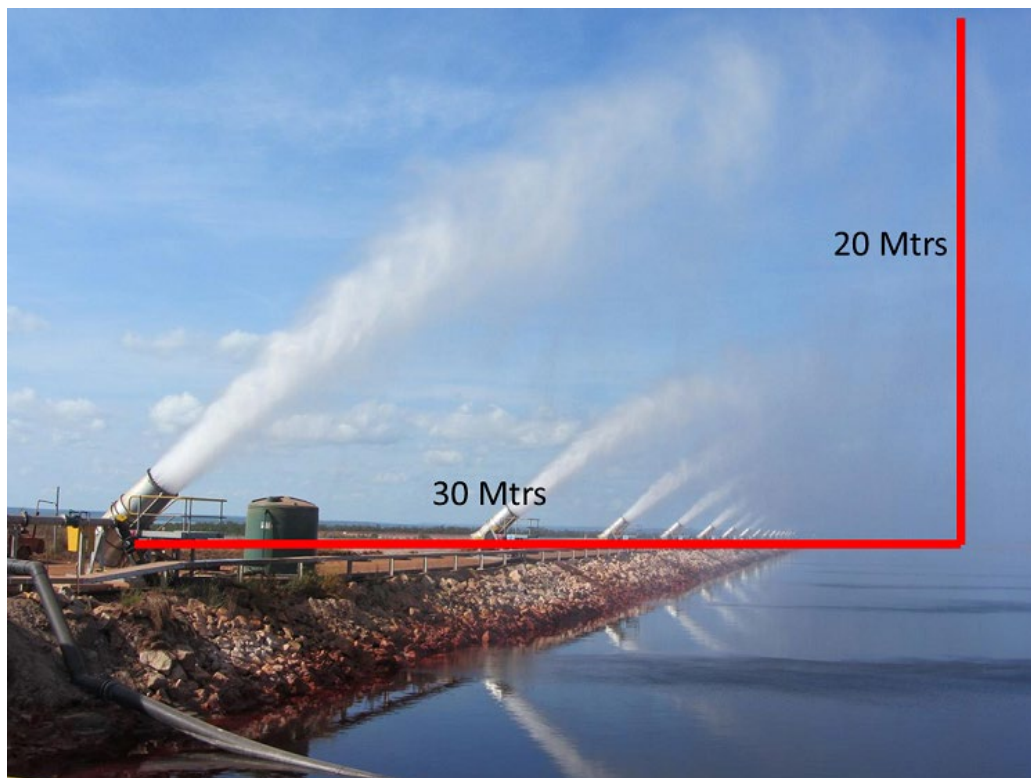
Figure 4: Example Spray from Evaporator Fan Operation (Minetek)
